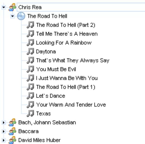
**Figure 6.64. Expanded `<rich:tree>` with child elements**
